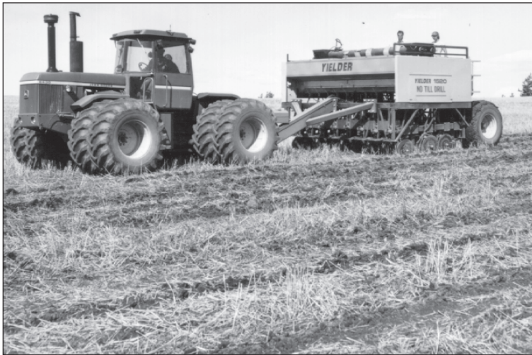
Figure 33.—No-till. Special drills allow planting directly into the standing stubble of a previous crop. By leaving the crop residue in place, more water is absorbed into the soil and much less runs off. Water saved increases crop yields, and reduced runoff lowers erosion substantially.
