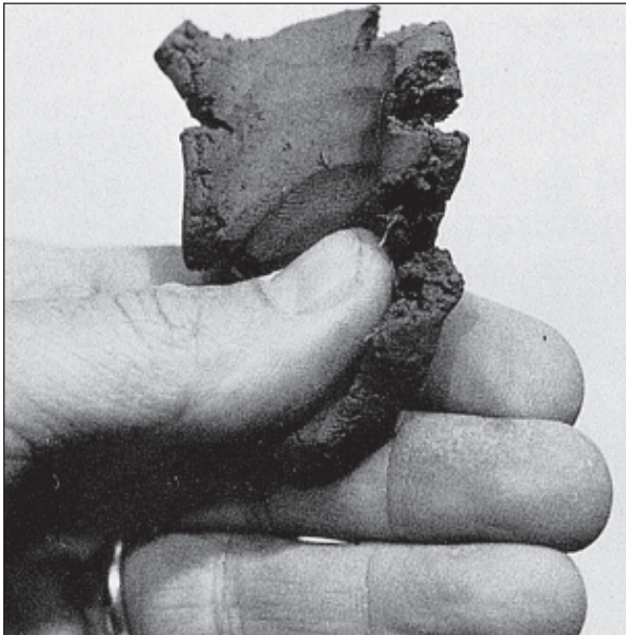
Figure 10.—Silty clay loam texture. This soil has 3 percent sand, 68 percent silt, and 29 percent clay. It forms a smooth ribbon about an inch long.
