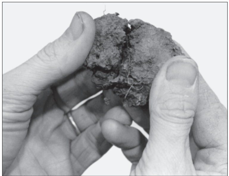
Figure 12.—Determining soil structure. Hold a clod of soil in both hands and apply gentle pressure. If the soil breaks easily along a natural plane of weakness, it is breaking into units of soil structure.
