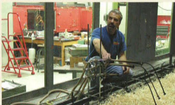
A Forest Service scientist sets up fuel and an ignition source to run an experiment in the Fire Lab's wind tunnel.
